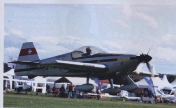
Swiss-built 2-seat, composite aerobatic trainer, the Votec 252T has a 250hp Lycoming
