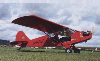
Let-Mont TUL-01 Tulak Piper ultralight seats just one, despite its resemblance to the Cub
